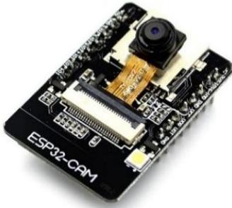
**Gambar 2.** Gambar 2.5 ESP32-CAM
