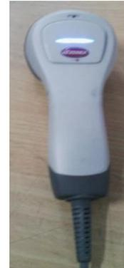
**Gambar 2** USB Barcode Scanner
