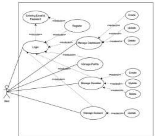
Figure 4. User Use Case Diagram
